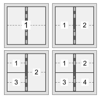
Figure 2: Channel assignment of wall transmitter module 1-gang, 2-gang, 3-gang and 4-gang
