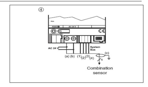
If possible, connect the shield of the combination sensor (yellowgreen, (c)) to earth potential (not to GND!). If this is not feasible, the shield must remain unconnected. When the shield is connected with GND, trouble-free operation of the device cannot be guaranteed.
