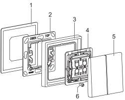
Fig. 1: Device components
