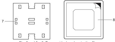
Fig. 2 and fig. 3: Transport lock and protective film
